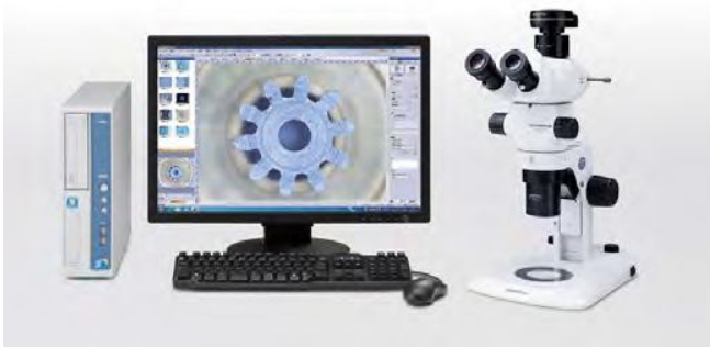
SZX7 in combination with DP26 digital camera system
