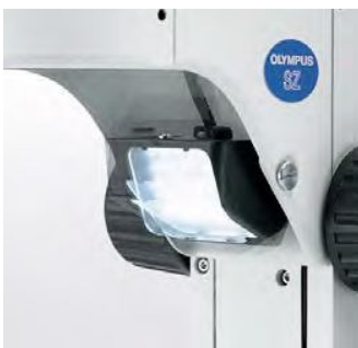
Flexible angle of LED light source
